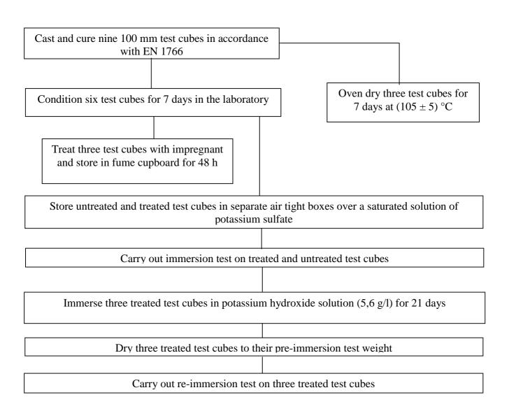
Figure A2.2: Flow chart of test procedure for absorption and resistance to alkali test
