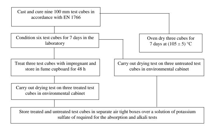
Figure A2.1: Flow Chart of Test Procedure for Drying Test
