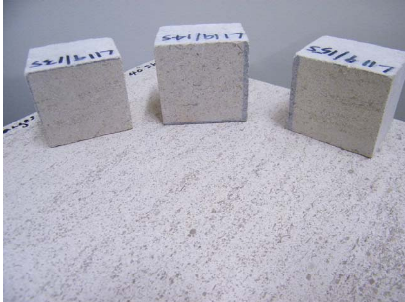
Plate 1: Appearance of Valanges limestone specimens treated with 40SK after the resistance to salt attack test. Specimens are compared with original finish of Valanges treated with 40SK.
