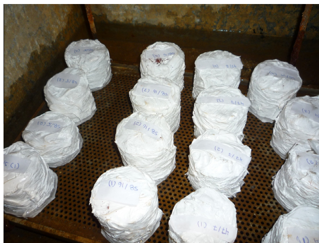
Fig. 6. Cores sealed with proprietary polysulphide sealant for capillary absorption testing.
