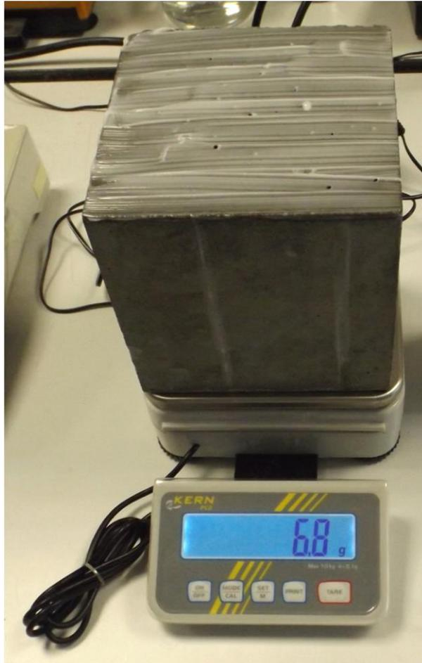
*Picture 1: Control of coverage rate by means of a balance*
